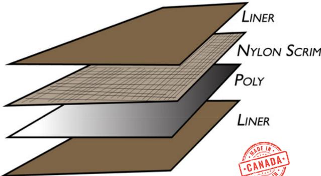
Jona Guard temporary surface protector is made with 4 ply technology offering advanced mud and moisture protection. Use to protect your floors during construction, renovation projects or while moving.
