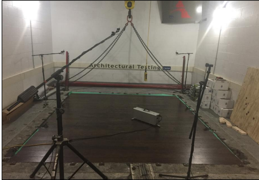
Source Room View of Test Specimen Installation
